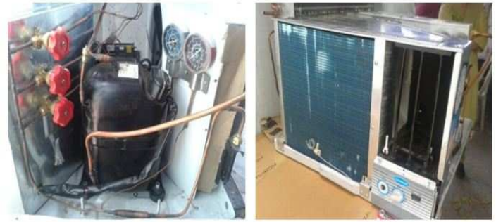
FIG:2a –Open Unit FIG:2b –Closed Unit Fig:2-Air Conditioner Experimental Test Unit
